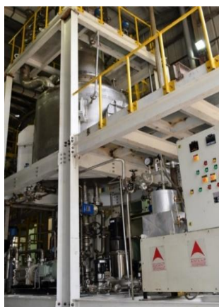
5 cu.m/d Brine Concentrator Unit
