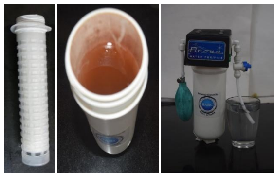
HF membrane cartridge; bottle with turbid water; filtered water collected after pressurizing
