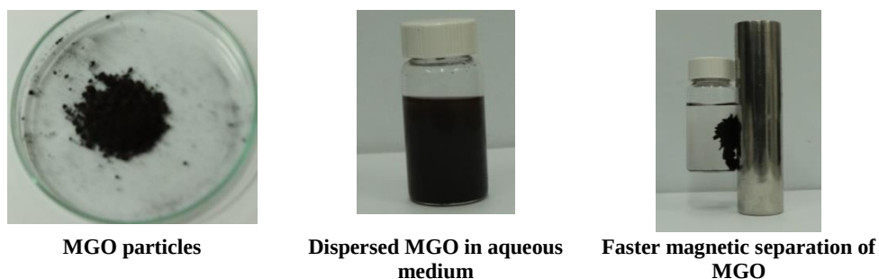
Fig. 5. Images of prepared MGO, dispersed MGO, and magnetic separated of MGO in the presence of external magnet.
