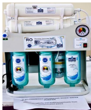
Brackish Water Reverse Osmosis Unit
