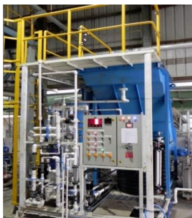
10 cu.m/d Brine Purification System
