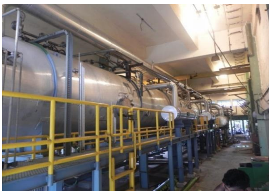
240 m 3 /day capacity MED-TVC plant at BARC
