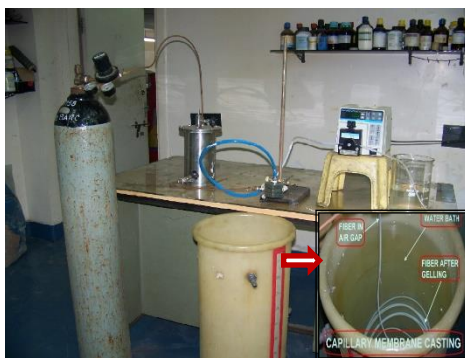
Fibre spinning set-up for hollow-fiber membrane preparation
